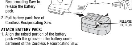
2. Press the battery pack into place. Make sure the latches are securely fastened. Do not use the Cordless Reciprocating Saw if the battery pack is not seated properly.
